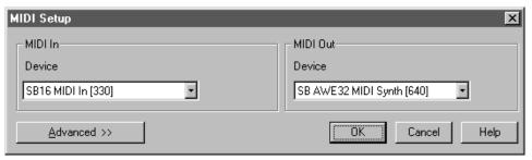
This diagram shows the MIDI Setup dialog box properly configured to play back through an external MIDI device. Keep in mind that the specific driver names will change depending on what sound card or MIDI device you have.
